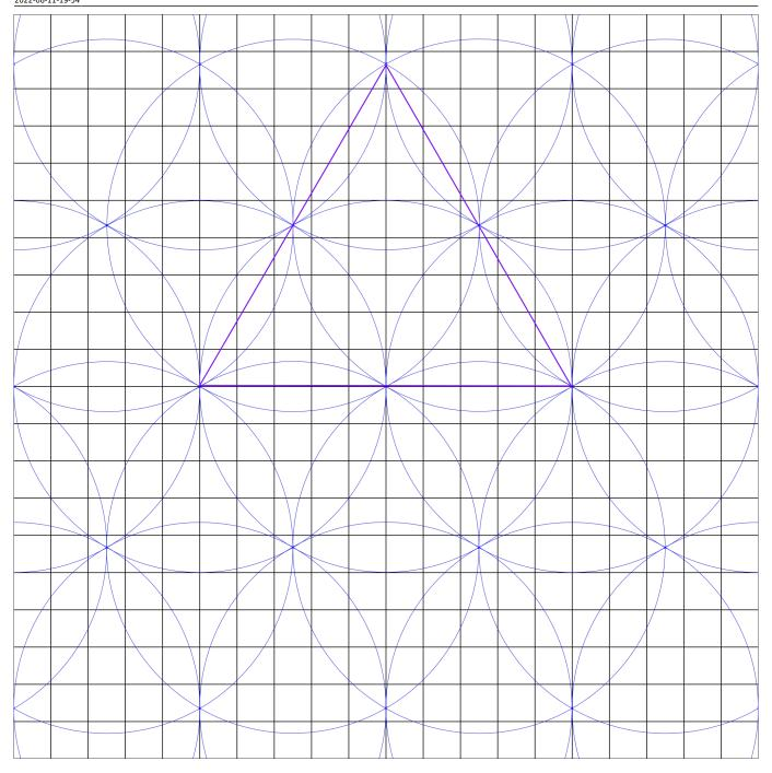
Considering the shown area (purple triangle) of  $1.3\times10^6$  and the average sensor stations placed there (\$2\$), the area covered by one station on average is  $0.65\times10^6$ . To have a comparison: A sole station as an area of  $3.1\times10^6$ . So there is roughly only one fifth of the effective area of each station used.
