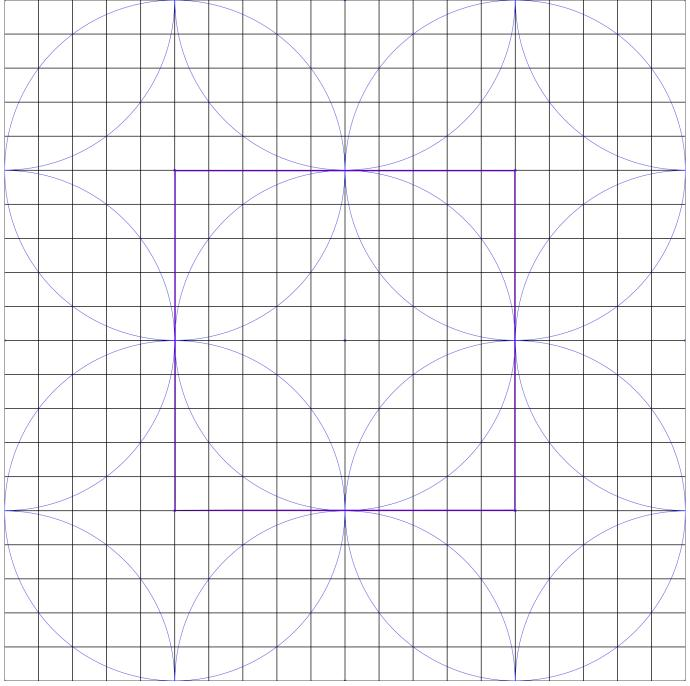
The enclosed area for this pattern is \$4\times10^6\$ and encloses \$2\$ stations on average. This makes the covered area per station \$2\times10^6\$. That's considerably better than the Maximum Redundancy pattern with 1.57 stations more for the same area. The biggest problem here is, already one station missing leaves a gap:
