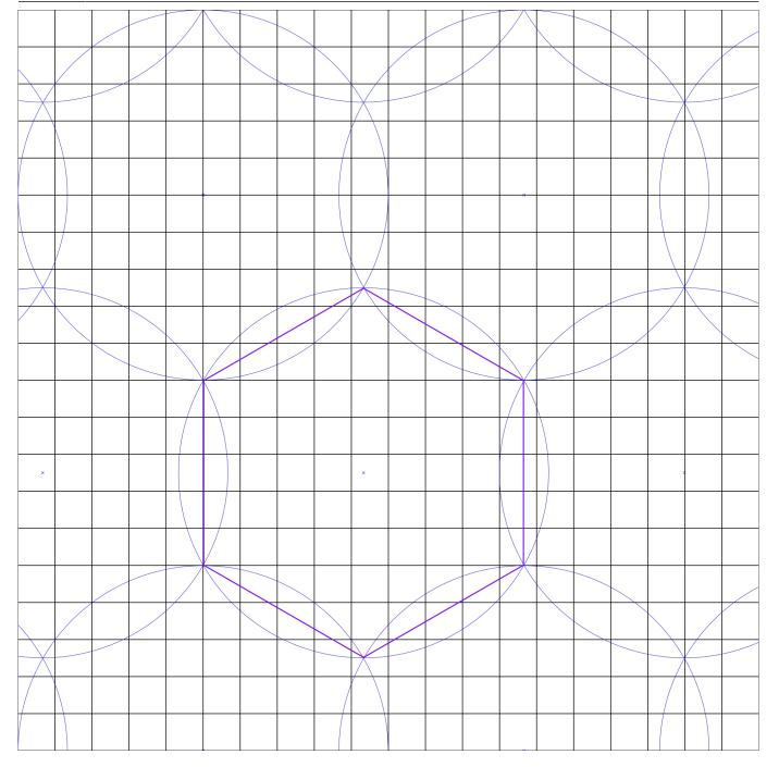
The purple area os such a hexagon is \$2.6\times10^6\$ encloses exactly one station, so the area per station is \$2.6\times10^6\$ or 83% of a sole station. It is very cheap to cover the entire map without leaving any gaps to slip through. The two problems with it are: The redundancy is practically non-existent:
